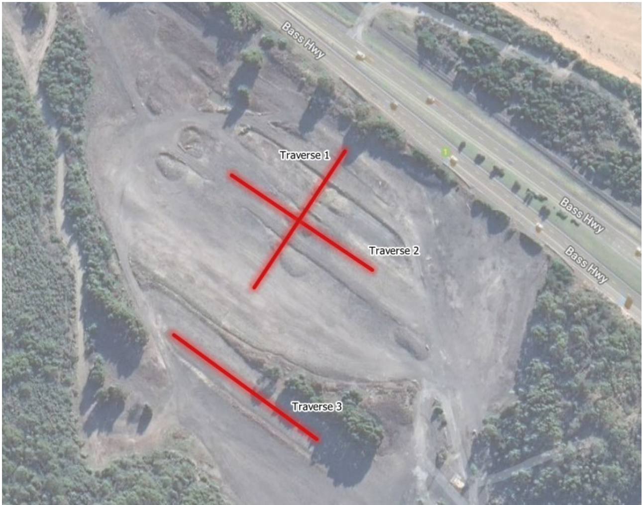
Figure 3-1. Electrical resistivity traverse locations (indicative)
