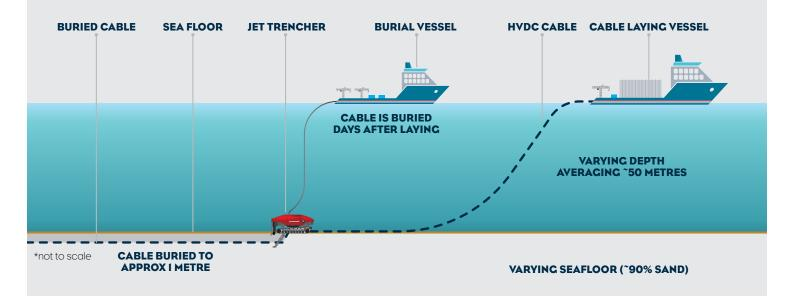
The majority of the subsea cable route has a soft, sandy seafloor, allowing a water jetting trencher to be used to safely bury the cables, with low impact to the surrounding environment
