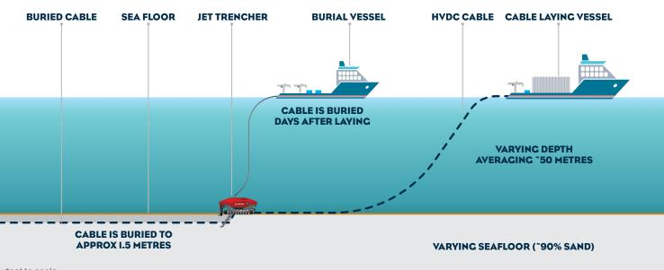
The majority of the subsea cable route has a soft, sandy seafloor, allowing for a water jetting trencher to be used to bury the cables safely and with a low impact to the surrounding environment
