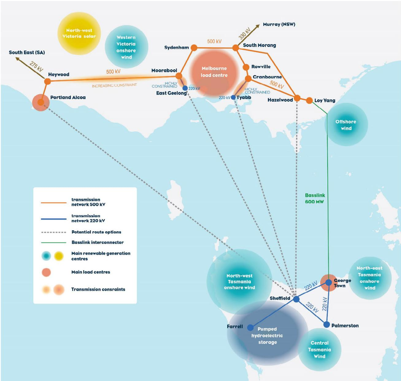
Figure 5-1 Potential grid connection points
