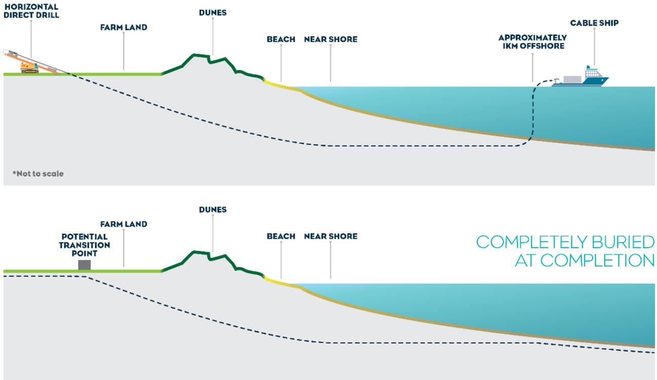
**Figure 8-8 Indicative Victorian shore crossing showing proposed horizontal directional drilling installation**
