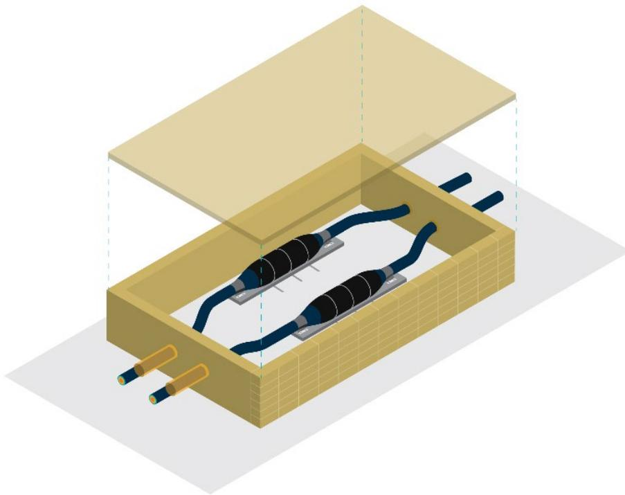
**Figure 2-3** Typical land cable joint bay (Source: Europcable)
