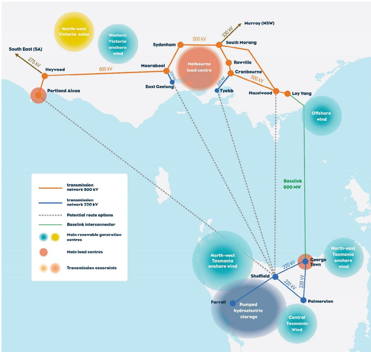
Figure 1-1 Strategic overview of potential grid backbone connection points
