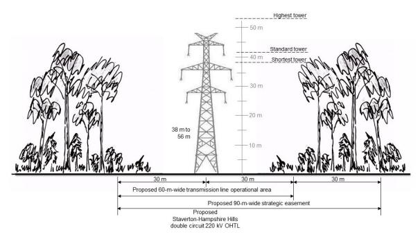
Figure 3-2 Conceptual arrangement of Staverton – Hampshire Hills easement and transmission line operational area from Cethana to Wey River (looking west from Cethana)
