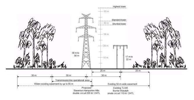
Figure 3-3 Conceptual arrangement of Staverton – Hampshire Hills easement and transmission line operational area from Wey River to Hampshire Hills (looking north from Wey River)
