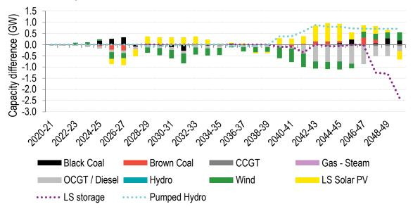
Figure 31: Change in NEM capacity due to Snowy 2.0 for EC90 and Marinus 600 MW (Snowy 2.0 EC90 with Marinus minus EC90 with Marinus)
