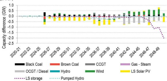
Figure 46: Change in NEM generation mix due to increased Marinus limit for EC90 (Marinus1200 EC90 with Marinus 1,200 MW minus EC90 with Marinus 600 MW; difference relative to sum of Figure 25 and Figure 28)
