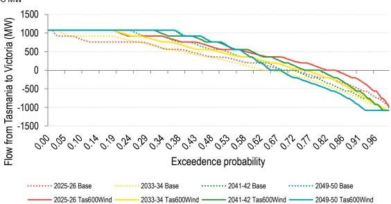
Figure 35: Duration curve for cumulative flow of Basslink and Marinus for Tas600Wind with Marinus 600 MW
