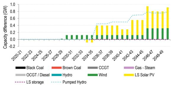
The change in Victoria's capacity mix with Marinus is shown in Figure 13, relative to the mix shown in Figure 9. These figures show that Marinus is only expected to defer a small amount of OCGT
