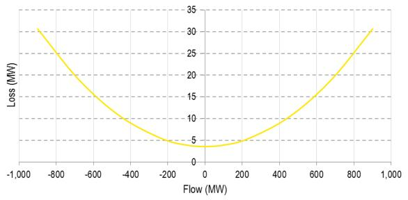
For the sensitivities that assume a 1,200 MW capacity for Marinus we have modelled two 600 MW capacity interconnectors in parallel using the same assumptions described above. This gives a total of 1,200 MW of additional interconnector capacity relative to the Basslink only counterfactual.
