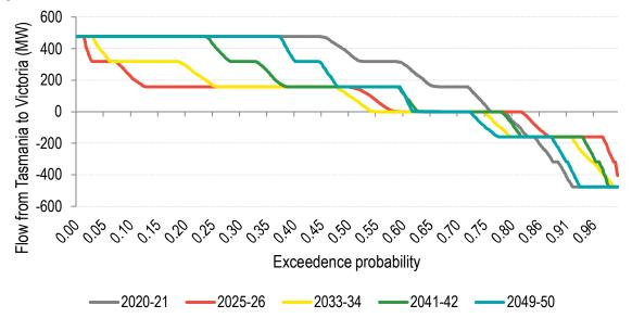
The forecast effect of Marinus in its first year of operation (2025-26) is to increase exports to the mainland over the evening peak from about 400 MW with Basslink alone to about 650 MW with Marinus and Basslink combined. Furthermore Marinus and Basslink combined import on average 100 MW to Tasmania during the day, whereas Basslink alone cannot store sufficient energy to allow daily imports. Marinus therefore allows greater arbitrage between Tasmania and the mainland than Basslink alone.
