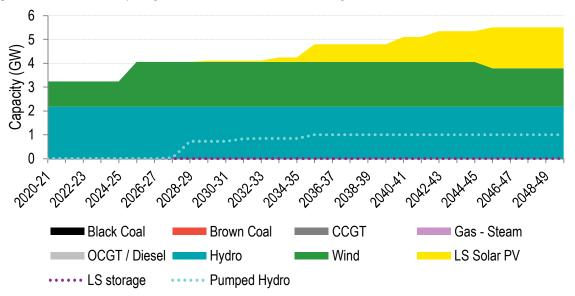
Figure 47: Tasmanian capacity mix forecast for EC90 sensitivity with Marinus 1,200 MW
