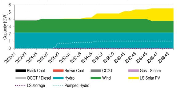
Figure 54: Tasmanian capacity mix forecast for EC90 Tas600Wind sensitivity with Marinus 1,200 MW
