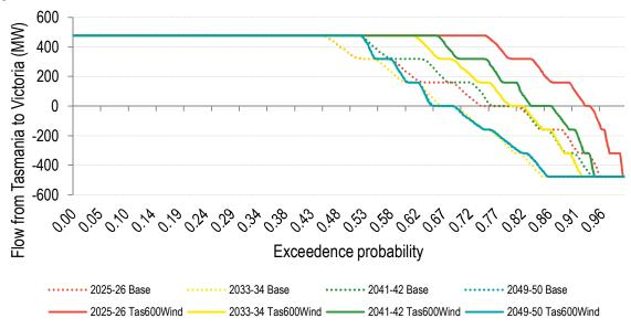
Figure 36: Duration curve for Basslink flow for Tas600Wind without Marinus
