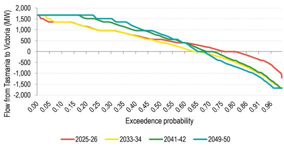
Figure 53: Duration curve for Basslink and Marinus 1,200 MW flow for Marinus1200 Tas600PSH Tas600Wind Scenario with Marinus
