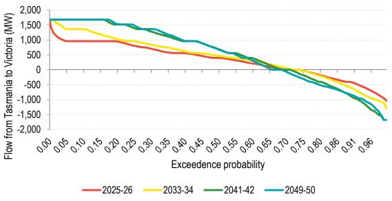
Figure 44: Duration curve for Basslink and Marinus 1,200 MW flow for Marinus1200 sensitivity with Marinus
