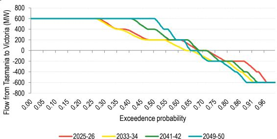
Figure 17: Duration curve for Marinus flow for Base Case with Marinus 600 MW
